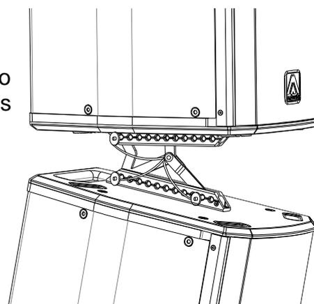
**Fig. 20.** Flying of two units X102FD with HR-L102
