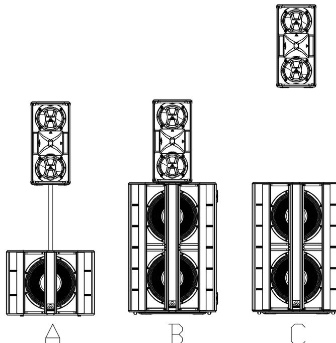
**Fig. 15.** X102FD with subwoofer (A: with pole, B: stacked, C: flown)
