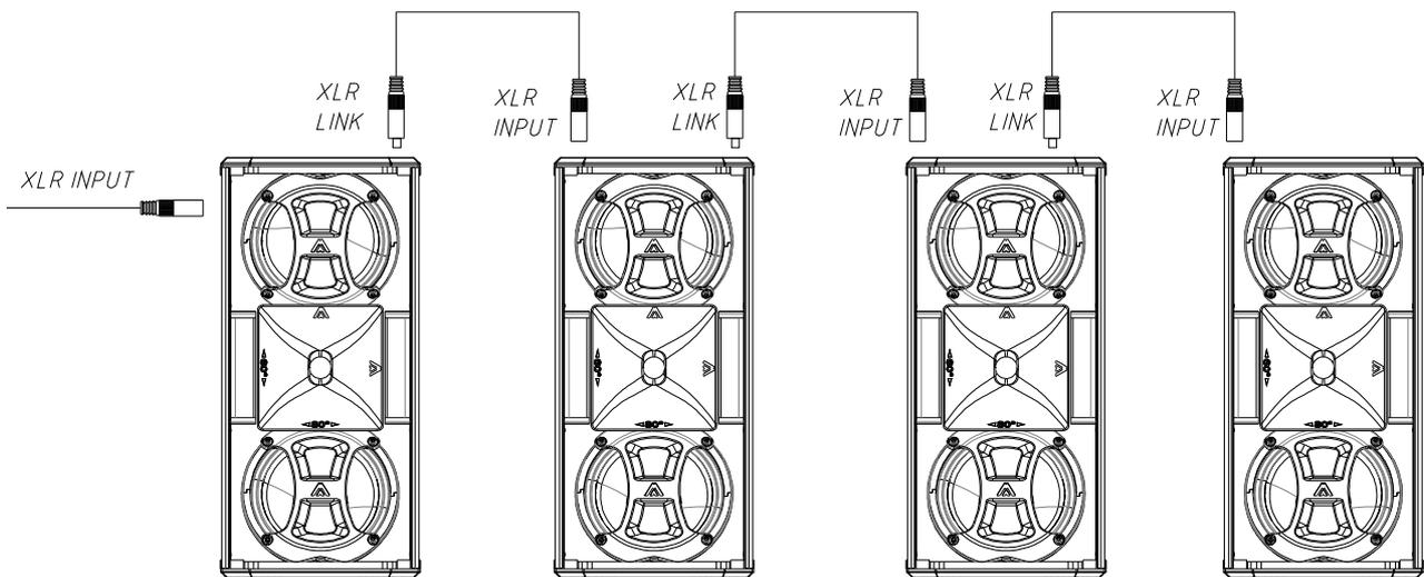
Fig. 7. Parallel connection for the X102FD (signal)
