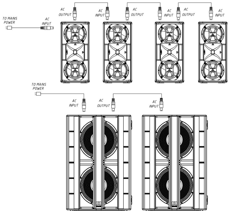
**Fig. 11.** Parallel connection for the X102FD and XW218 (mains). Do not connect more than four units of X102FD or two units of XW218 using the AC Mains link connector.
