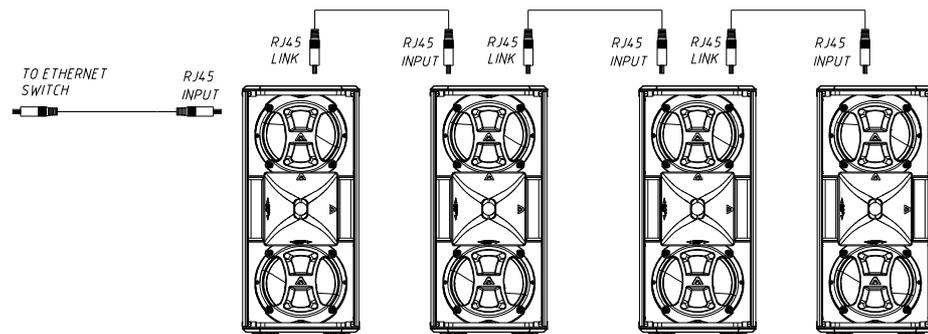
**Fig.12.** Parallel connection for the X102FD and XW218 (network). Do not daisy-chain more than eight units of each when using Dante networking (as in the diagram).
