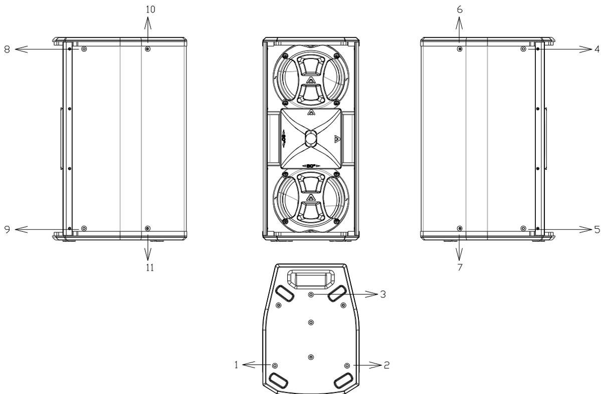
**Fig. 17.** X102FD horizontal and vertical flying points
