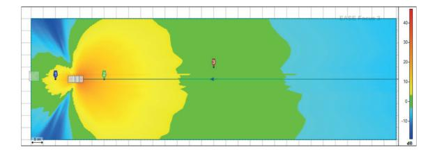
Notice that the end-fire is not a preset, so now we need to apply the corresponding delay in each subwoofer. Set the preset to the default one
