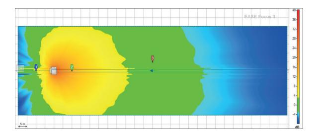
Looking the coverage response we can see clearly how now that there is a valley of sound pressure level on the rear part (receiver #1), with an increased SPL in the near-field (receiver #2).
