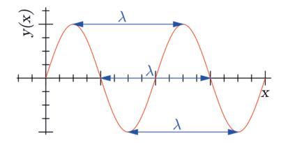
**The phase (θ)** of a signal is the relative time shift of this signal with another one used as reference.
