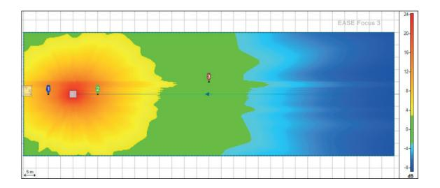
We can see in the simulation how indeed the three subwoofers directivity is omnidirectional. Looking at the frequency distribution chart also we can see how when increasing frequency the array is more directional, but it won't affect our system due the low pass filter of the LPF80 preset.
