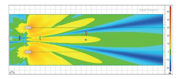
Though is this effect is not that noticeable in the frequency distribution chart, it is well shown in the venue simulation how at 50 Hz we get "corridors" with no SPL.
