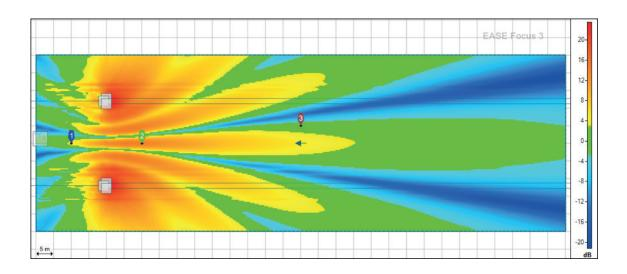
We get exactly the same effect. In all stereo subwoofer configurations we get odd frequency response. In terms of sound quality, these configurations should never be used.
