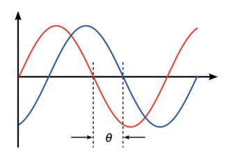
The phase is measured in radians or polar degrees. 180 polar degrees are the same as  $\pi$  radians. With the previous phase between two equal sinusoidal signals, this means the peak of one signal would be matching a valley of the phased version, so when summing both signals the result is no signal (destructive interference).
