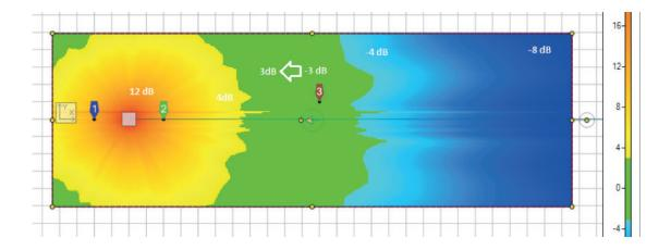
The relative sound pressure level representation is a bit harder to understand but very useful. Here what EASE Focus 3 is doing is assign the green colour to the zones where the SPL is 3 dB above or below the mean SPL in the entire venue (the ideal target). Warmer colours are assigned to the zones with more than a +6dB of deviation from the mean SPL so zones with a very high of sub bass presence. Colder colours are assigned in the zones where the SPL decays.
