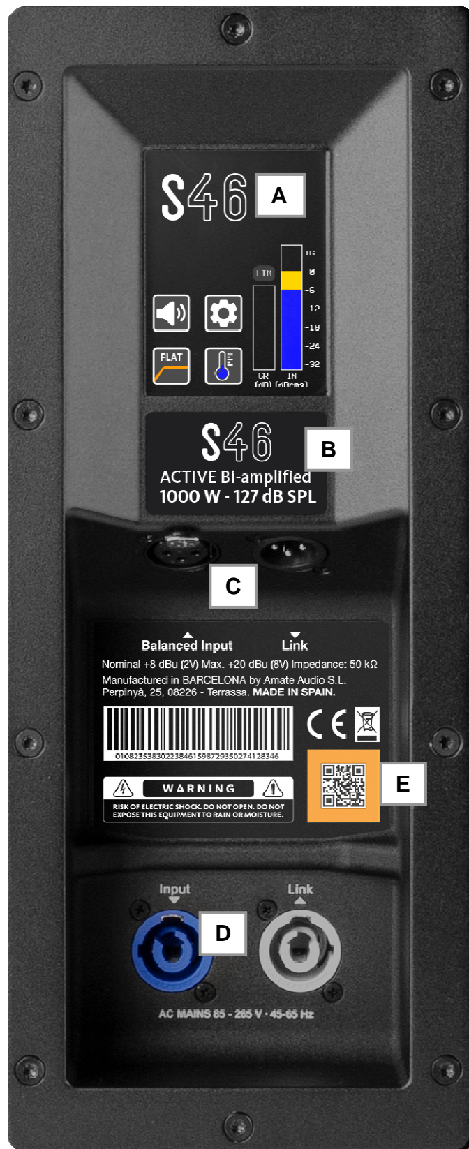
Fig. 2. S46 control and connection panel
