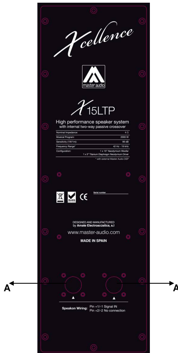
Fig.11. X15LTP connection panel
