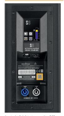
Amate Audio's latest generation DSP System management is integrated with 3rd generation Class D amplification. Colour touchscreen operation and monitoring of DSP System includes access to powerful presets - engineered by Amate Audio R&D team – that instantly configure your Nítid loudspeaker for the majority of common application environments within seconds, prior to rigging or installation.
