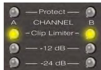
**| Make sure this LED is not alight permanently !** No extra power is obtained in this way losing dynamics and sound quality.
