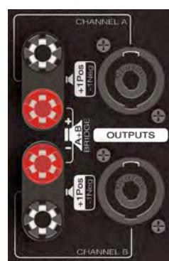
There are two speaker outputs: CH A and CH B both fitted with Speakon sockets and Terminal type (binding posts) connectors.
