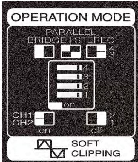
To use Bridge mode, place the DIP switch 3 and 4 ON. The corresponding indicator located on the front panel will light up (BRIDGE). The amplifier gain will be controlled exclusively by CHA gain potentiometer.
